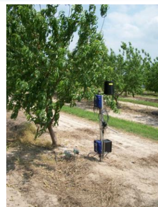
Figure 1 - Field Station automatically measuring and transmitting tensiometric soil moisture and other soil indices at various depths.
