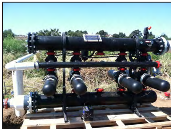
Figure 2. Example of a Netafim Apollo Disc-Kleen Filter
