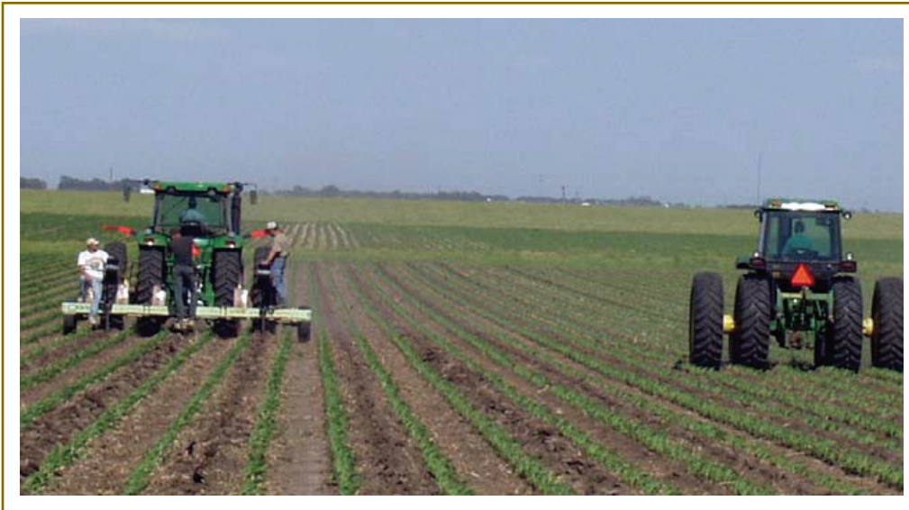
FIGURE 1 Tractor on left installing thinwall dripline while tractor on right packs soils left open by shank.
